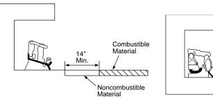
Figure 8 - Minimum Fireplace Clearances If Installed at Floor Level
